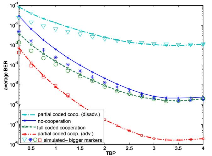
Fig. 9. Performance of the four cases of coded cooperation at  $\bar{\gamma} = 7.5\text{dB}$ : truncated bounds and simulation results. Partial cooperation is advantageous or disadvantageous from the point of view of one MS. Code-rate  $R = 1/3$ .
