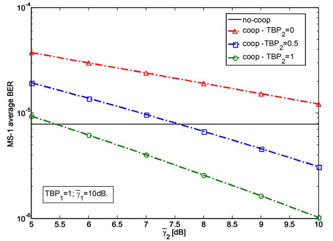
Fig. 8. Performance of MS-1 for asymmetric uplink channel conditions: MS-1 moves with  $\text{TBP}_1 = 1$  and  $\bar{\gamma}_1 = 10\text{dB}$ ; MS-2 moves at different velocities with varying  $\bar{\gamma}_2$ . Full coded cooperation and no-cooperation are compared. Code-rate  $R = 1/4$ .
