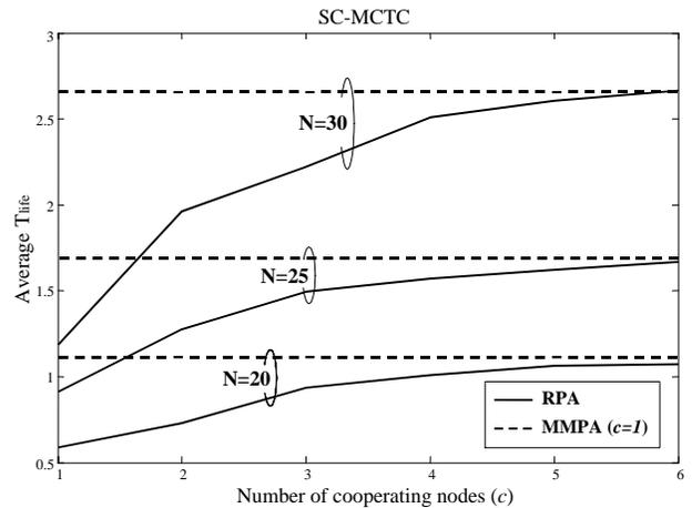
Fig. 6. Lifetime performances for varying number of nodes ( $N$ ) of an SC-MCTC with RPA (solid lines) power allocation strategy with respect to the number of nodes ( $c$ ) cooperating with the source. MMPA allocation with  $c = 1$  is shown as reference (dashed lines).
