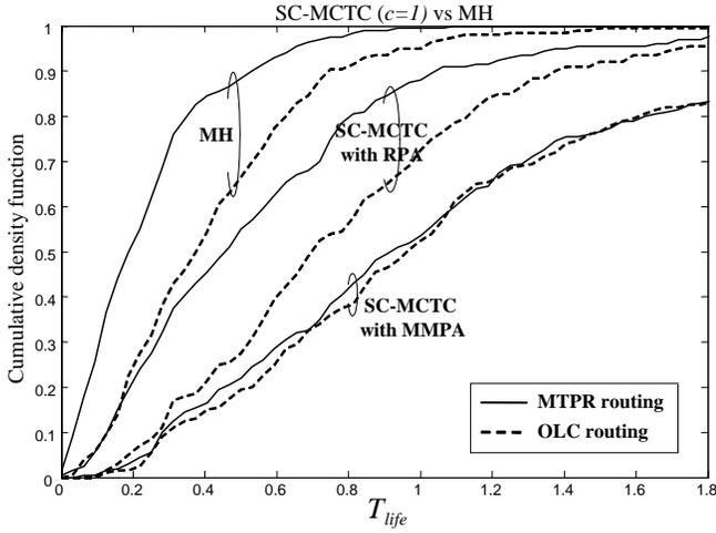
Fig. 4. Cumulative density function for the normalized network lifetime  $T_{life}$  for MTPR routing (solid line) and OLC strategy (dotted line) of the proposed MCTC with selection diversity (SC-MCTC) with recursive (RPA) and min-max (MMPA) power allocation schemes. The non-cooperative MH is shown as reference.
