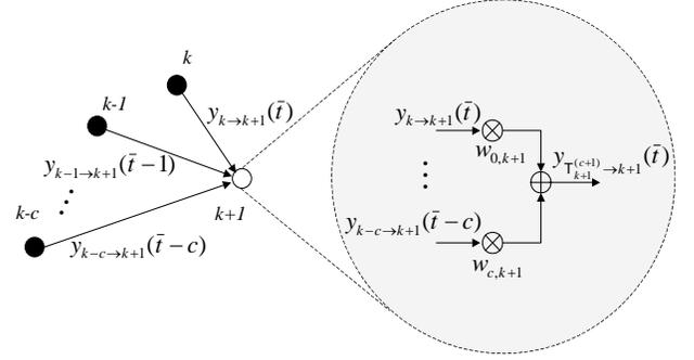
Fig. 2. Cooperating set of nodes relaying copies of the message  $x_S$  and the linear combining at the  $(k+1)$ th node (shaded area).
