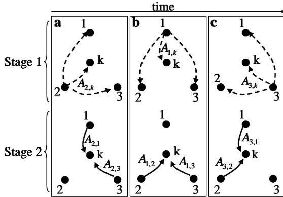
Fig. 3. Message exchange during link state estimation for 3 nodes that belong to the neighbor set  $N_k = \{1, 2, 3\}$  of node  $k$
