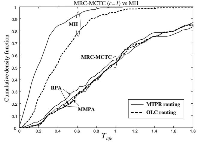
Fig. 5. Cumulative density function for the normalized network lifetime  $T_{life}$  for MTPR routing (solid line) and OLC strategy (dotted line) of the proposed MCTC with maximal ratio combining (MRC-MCTC) with recursive (RPA) and min-max (MMPA) power allocation schemes. The non-cooperative MH is shown as reference.
