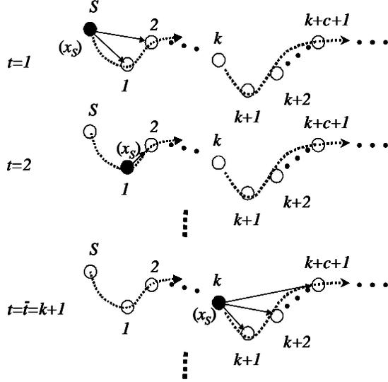
Fig. 1. MCTC timing and propagation of the transmitted message  $x_S$  (filled marker).
