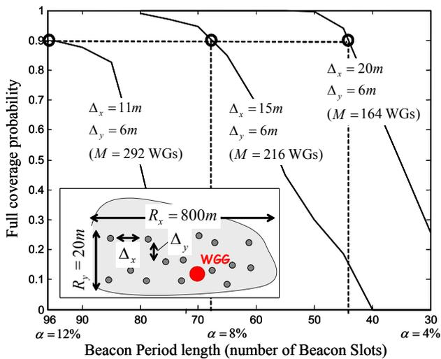
Fig. 5. Probability of full network coverage versus the length of the Beacon Period. Different acquisition geometries are considered ( $\Delta_x = 11m, 15m, 20m$ ) with  $\Delta_y = 6m, R_x = 800m$  and  $R_y = 20m$ .
