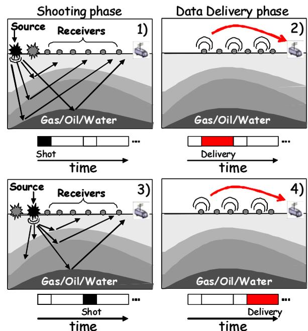
Fig. 1. Land seismic acquisition. Seismic waves are generated at surface by sources that are activated on different times and locations, elastic waves are back-scattered from sub-surface and are received by geophones. For every shot geophones recordings are delivered to the storage unit.
